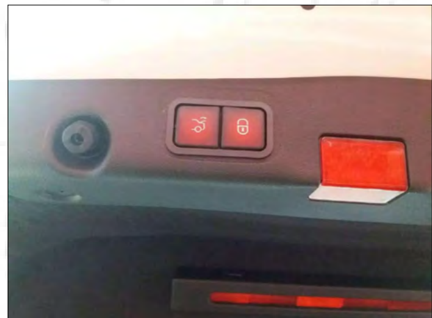
25. Install the tailgate switch button.
