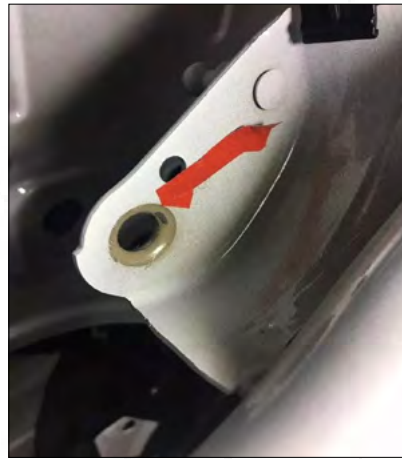
8. Remove the left spring and take out the spring hook film (The left and right steps are the same)
