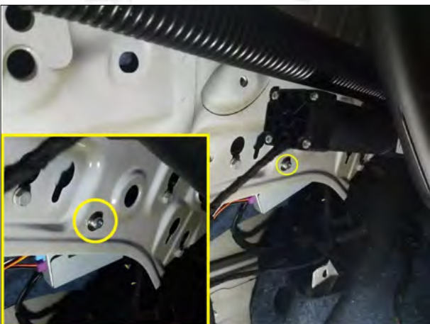
24. Install the central control box and fix it with the screws.
