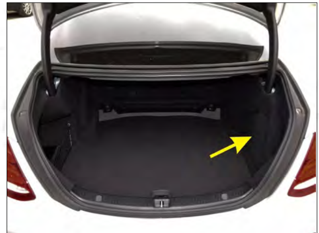
14. Remove the original car lock frame, as shown in the figure, our electric suction lock frame is installed at the position of the yellow circle.
