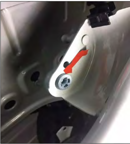
8. Remove the left spring and take out the spring hook film (The left and right steps are the same)
