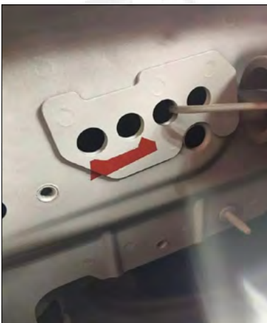
6. Put a rivet on the red mark hole on the left side of the trunk (The left and right steps are the same).
